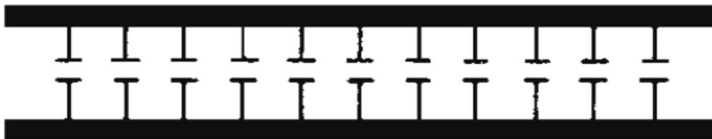
Figure 1-11.—Distributed capacitance.
